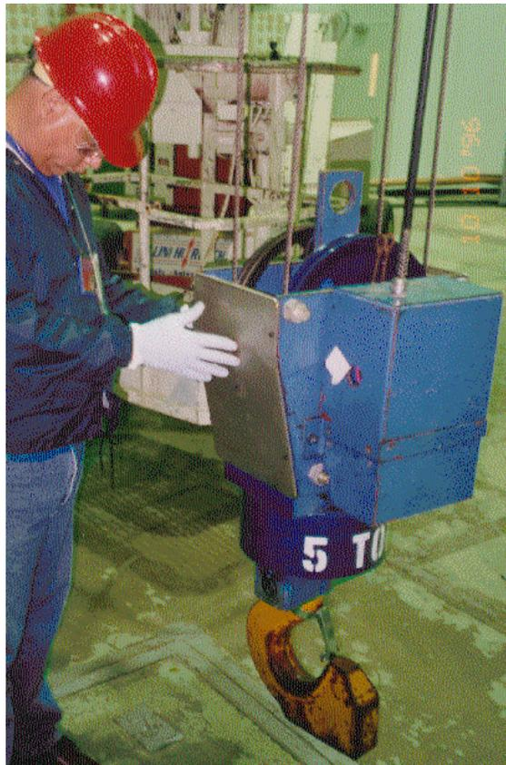
Figure 2. Electrically powered 5-ton rotating hook
