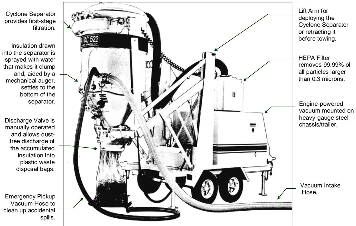
**Figure 6. VecLoader® HEPA VAC 522™ insulation removal system.**
