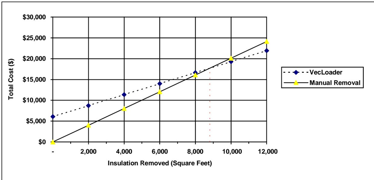
**Figure 7. Break-Even Analysis:** Although the unit cost of insulation removal is lower for the VecLoader, the total cost of using this technology is higher for job sizes less than 8,800 ft<sup>2</sup>. This is due to the higher fixed costs (\$6,077) of mobilizing and demobilizing the VecLoader. For job sizes less than 8,800 ft<sup>2</sup>, it is more cost-effective to remove insulation manually.
