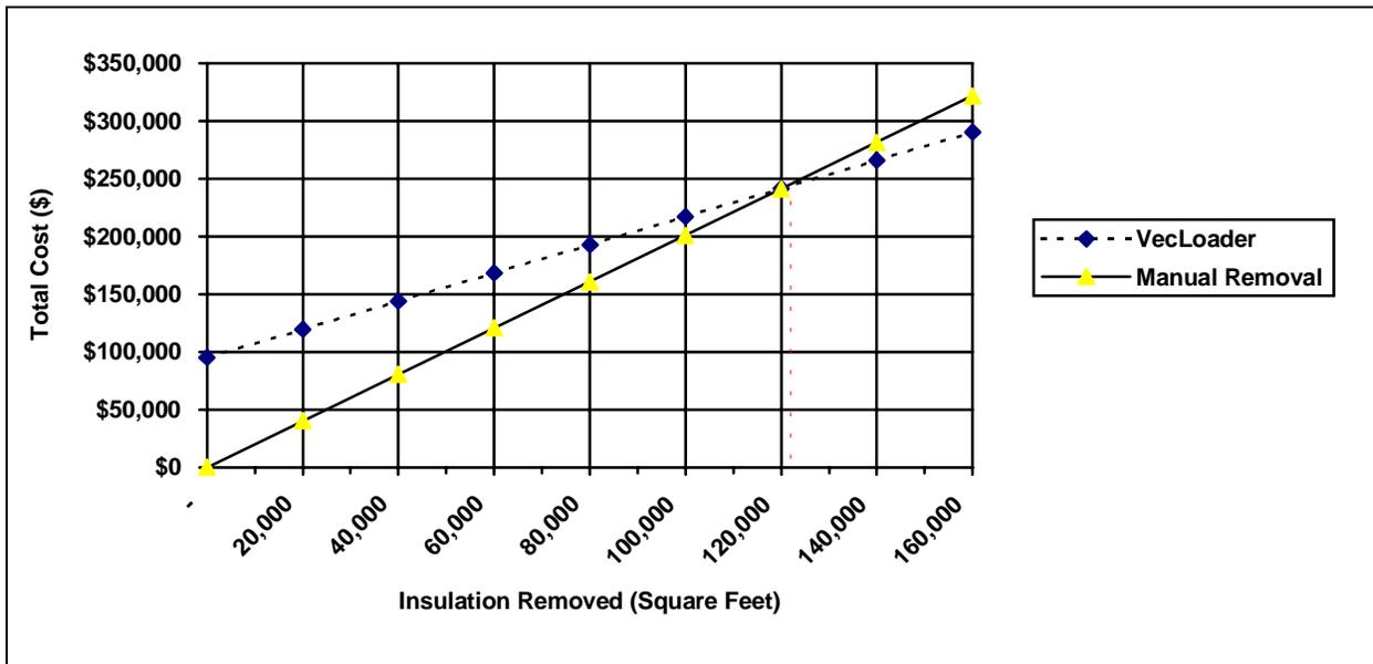
**Figure 8. Capital Cost Recovery Analysis:** The capital cost and fixed costs of the VecLoader are recovered after removing approximately 120,000 square feet of 4-inch insulation. If a project is estimated to have less than this amount of insulation, it may not be cost-effective to purchase a VecLoader for this purpose.
