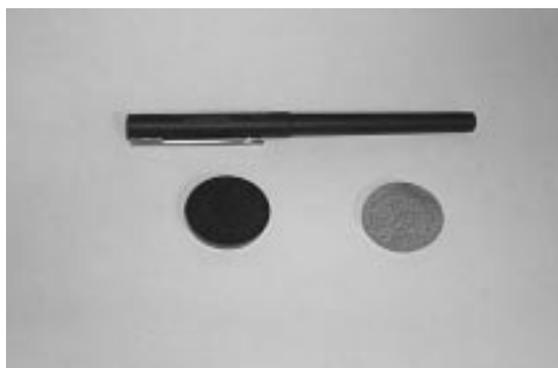
Figure 4. Samples Pressed into Pellets for Analysis
