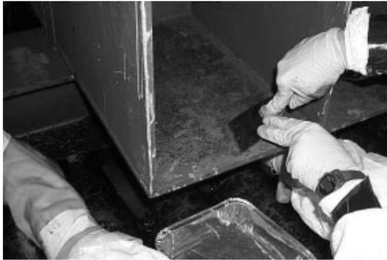
Figure 6. Collection of Paint Samples at TRA Delay Tanks.
