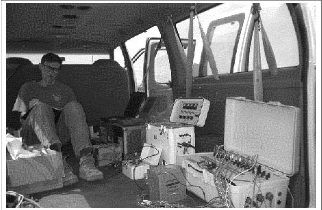
Figure 4. The field operations center for an Electrical Resistance Tomography For Subsurface Imaging network is typically located in a van or truck. A fast laptop computer can be programmed to process the data collected into two- or three-dimensional tomographs for site investigators to use on-site. Once the subsurface electrode arrays are emplaced and the network is set up, it can be run by a technician or put in automatic mode.
