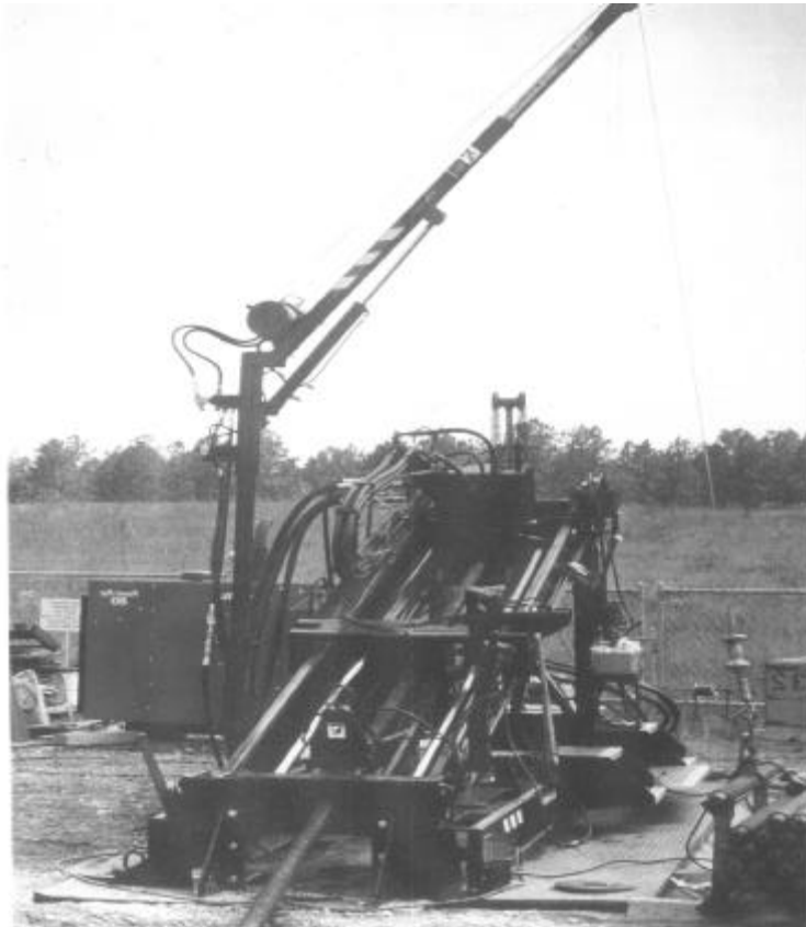
Figure 2. The Charles Machine Works prototype X-810 drilling rig tested at SRS.
