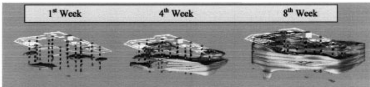
Figure 3. Progression of heated zone during thermally enhanced remediation
