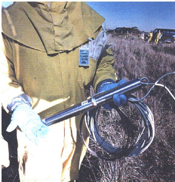
**Figure 3. Oxford Nanoprobe Assembly with NaI(Tl) Scintillator.**
