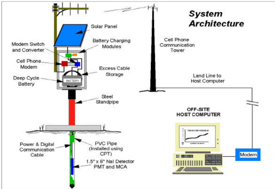
**Figure 2. Long-term Post-closure Radiation Monitor System (LPRMS) Architecture.**
