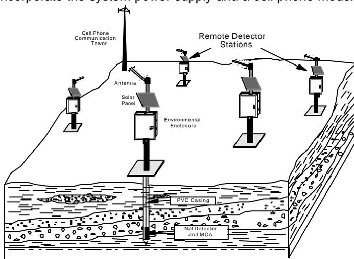
**Figure 1. Conceptual Drawing of Installed System**
