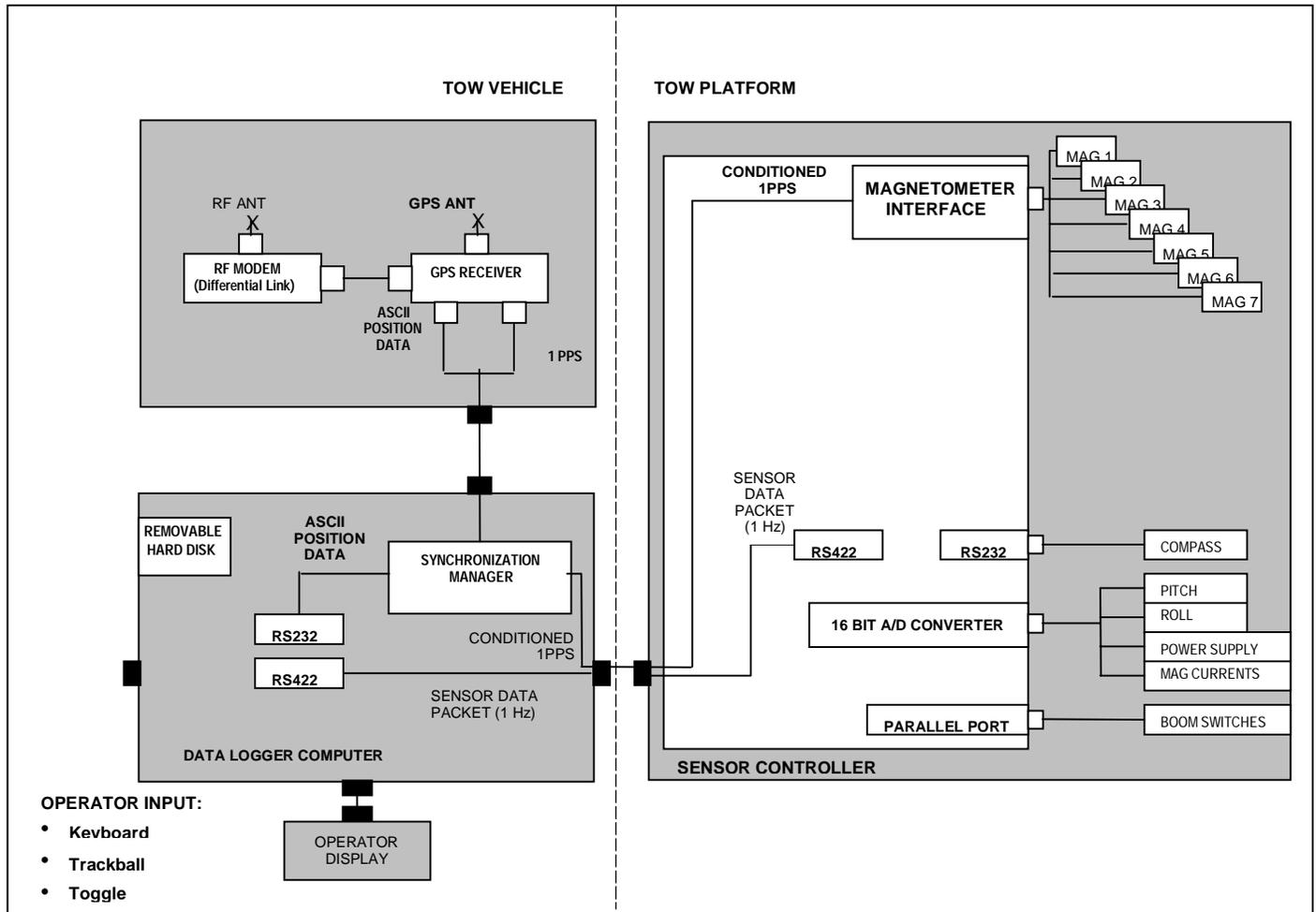
Figure 2. Schematic of Magnetometer Towed Array System
