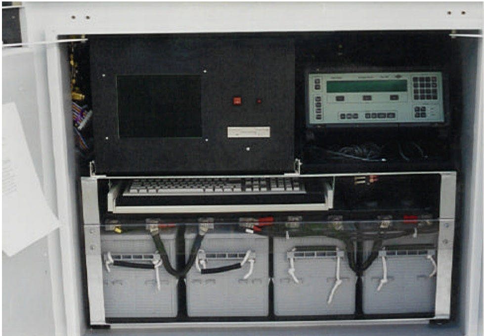
Figure 3. On-Board SEAtace™ Scanning System Components Protected in Environmental Enclosure
