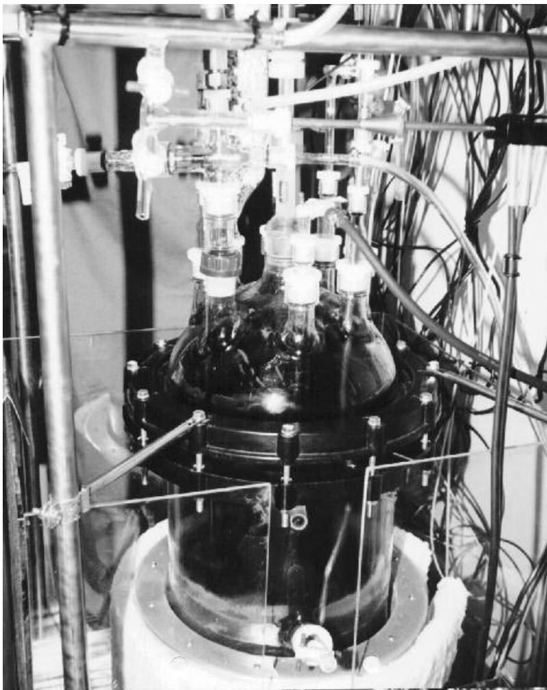
Figure 2. 40-liter Glass Acid Digestion Pilot Scale Reactor.
