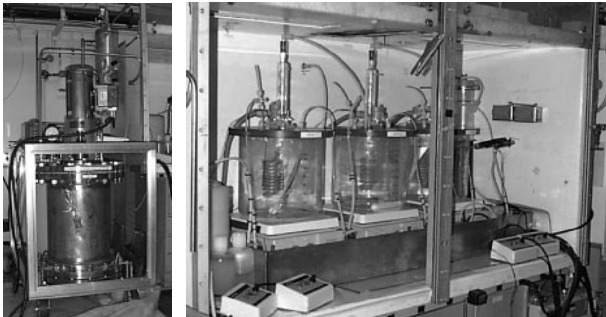
Figure 4. Pilot-scale laboratory unit used in destruction of trichloroethane (TCA) solvents, 15 kg/day. The 60-L hydrolysis vessel (left) converts TCA into water-soluble species, which are oxidized in a three-stage continuously stirred test reactor (CSTR) system (right). Data from this system are presented in Table 6.
