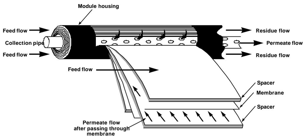
Figure 2. Schematic of a spiral-wound membrane module.
