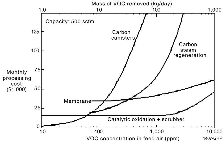
**Figure 6. Processing costs as a function of VOC concentration in a 500-scfm air stream for a membrane system and for competing technologies.**
