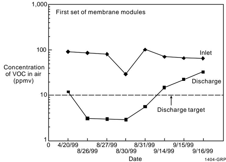
**Figure 4. VOC concentration in the membrane system inlet air (the SVE off-gas) and in the system discharge stream.**
