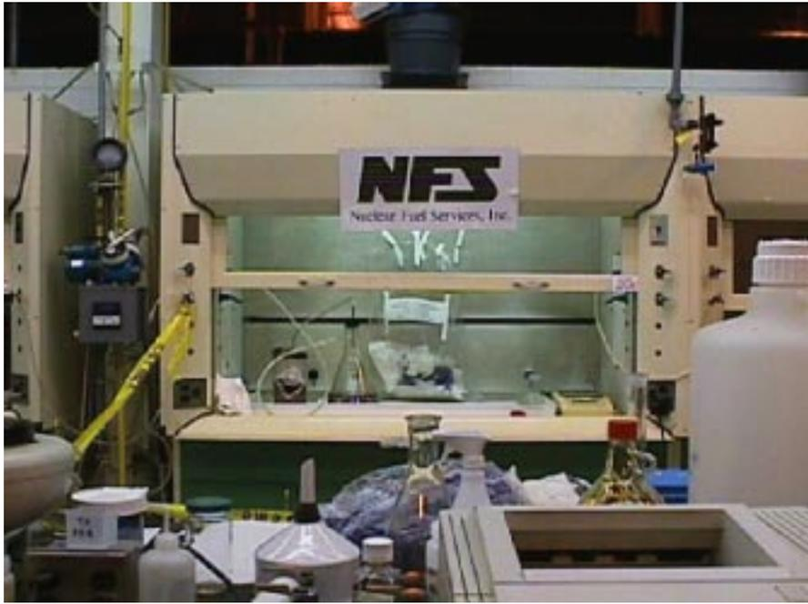
Figure 1. Photograph of equipment based in a ventilation hood for the DeHg process.
