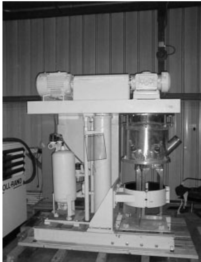
Figure 4. Planetary drum mixer for the deployment of mixed waste stabilization using CBPC.
