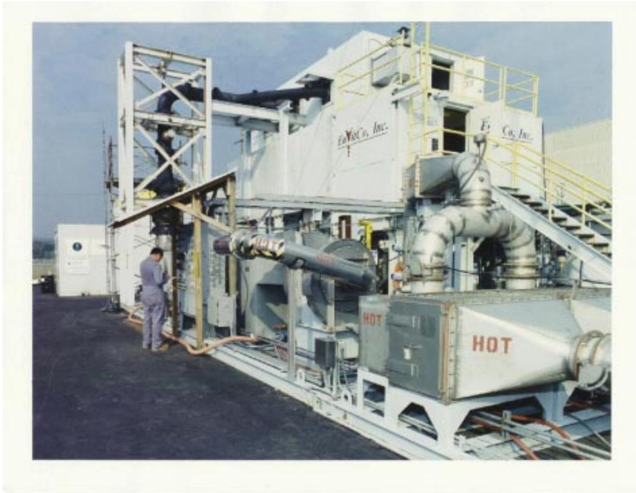
**Figure 5. Transportable Vitrification System (TVS) Melter with the Off-gas Emission Control Module in the foreground.**
