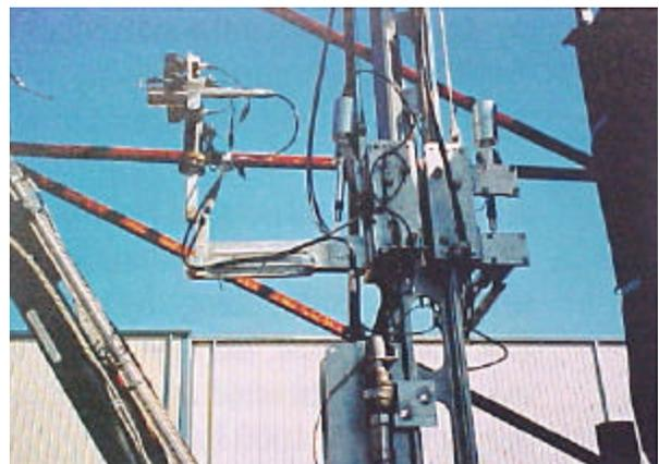
Figure 3. Camera assembly installed on mast.
