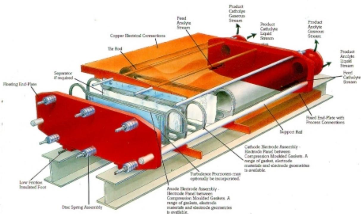
Figure 1. ICI FM21-SP Plate and Frame Flow Cell used in pilot-scale demonstration.
