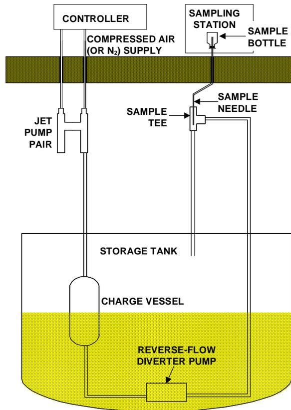
**Figure 3. Schematic of Fluidic Sampler technology.**
