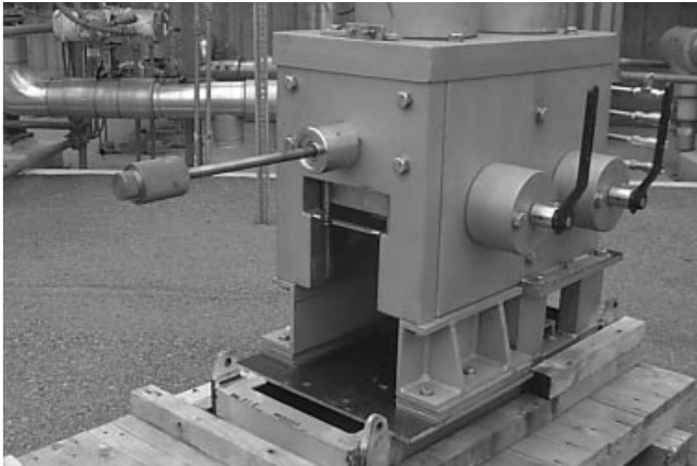
Figure 1. Fluidic Sampler bottle-handling apparatus sitting atop riser.
