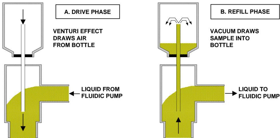
Figure 4. Sample bottle and needle detail.
