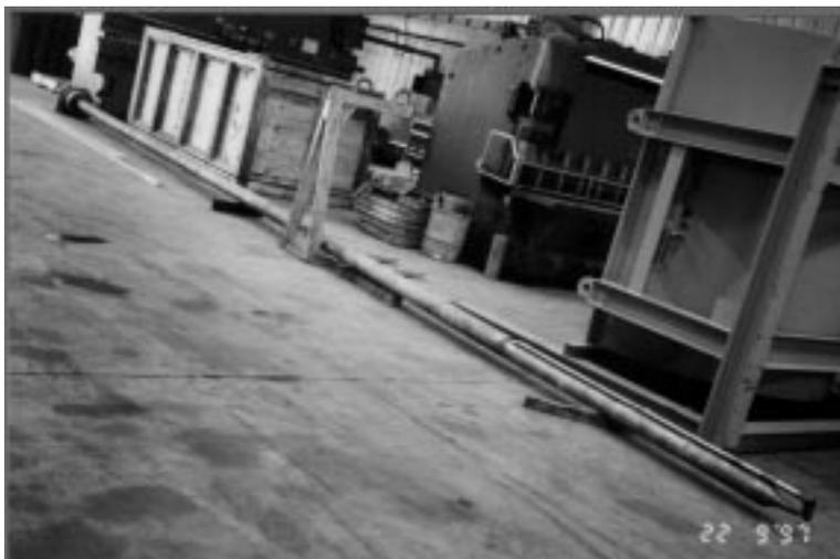
**Figure 2. Replacement plug and in-tank sampler pipework.**
