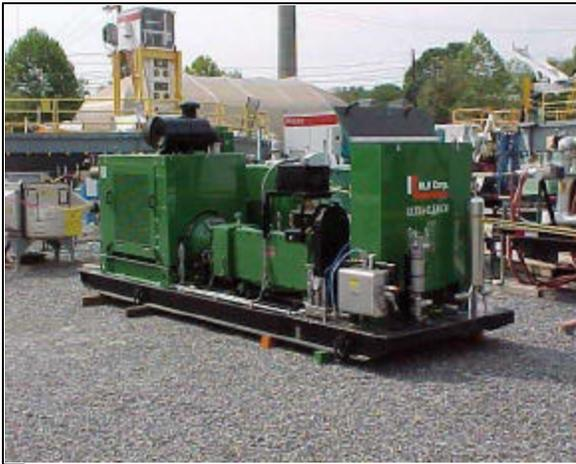
**Figure 4. Ultrahigh-pressure pump skid.**
