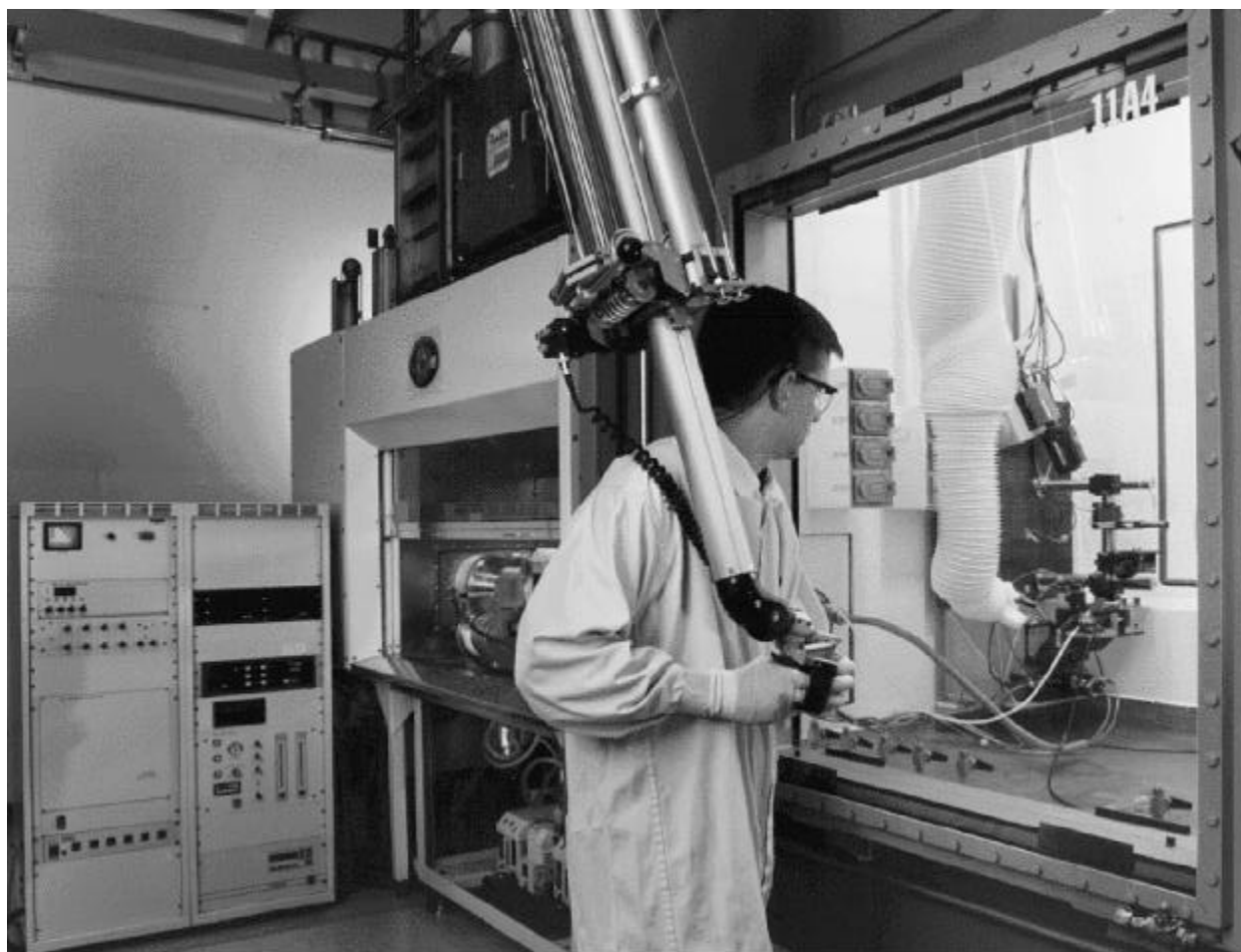
Figure 1. Laser Ablation/Mass Spectrometer (LA/MS) system showing in-cell equipment, operator with manipulator, fume hood, and electronics.
