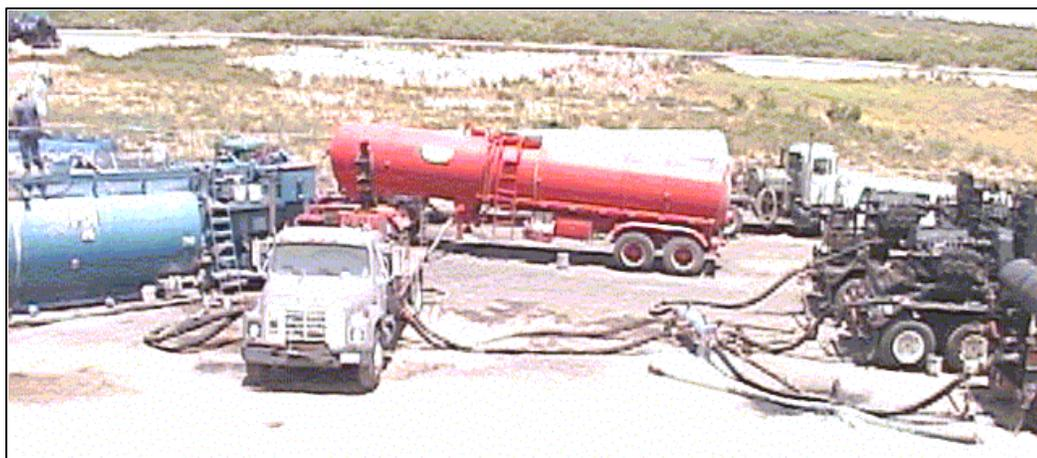
**Figure 2. Mobile grout plant used for 1999 field demonstration.**
