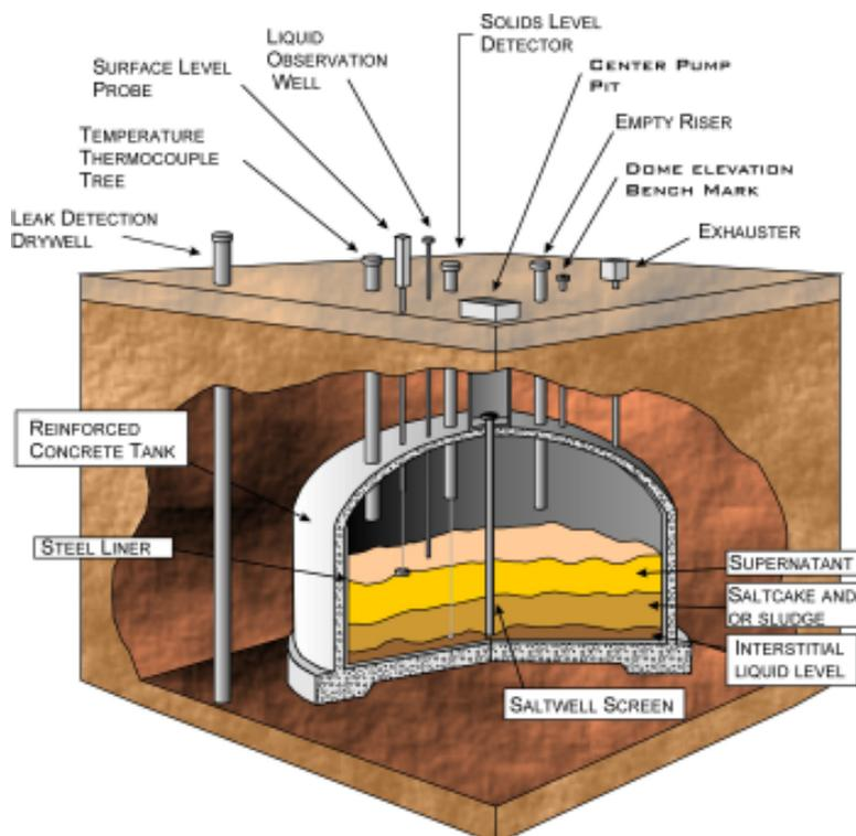
Figure 3. Example of a "typical" single-shell tank.
