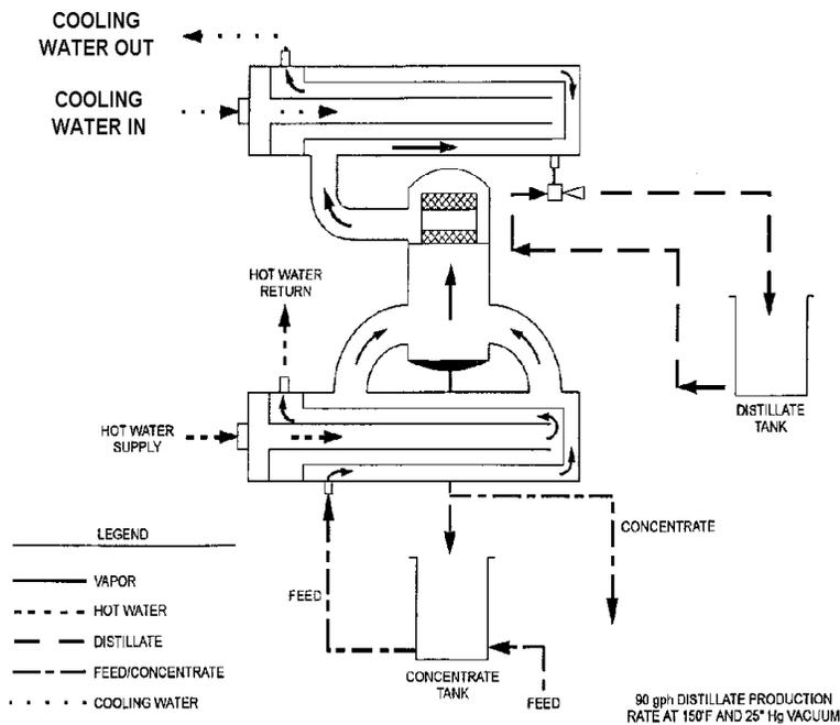
Figure 2. Basic flow diagram of the Out-of-Tank Evaporator.
