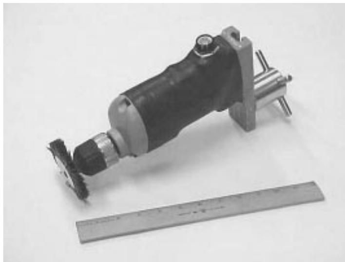
**Figure 3. Pipe Cleaning Tool.**
