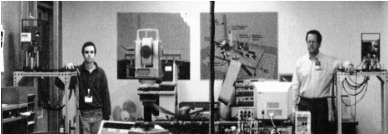
Figure 13-POTS Calibration. Two pods are shown on extreme left and right and theodolite in foreground.
