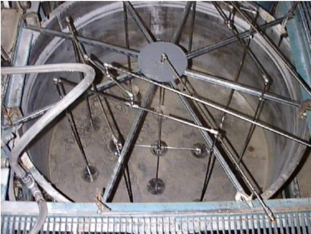
Figure 2. Pulsed-air mixing array in 1/12-scale tank (FY95) .
