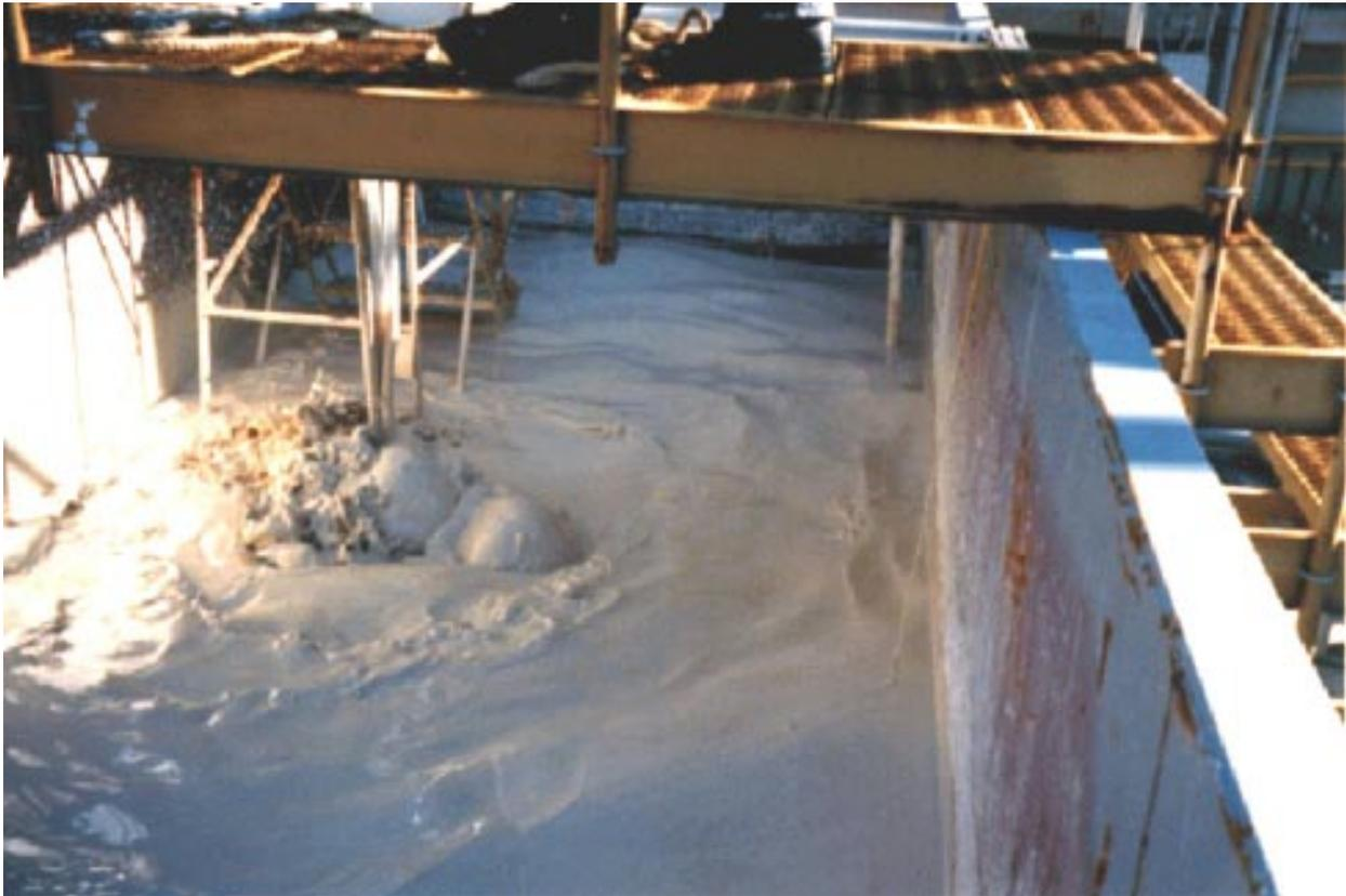
**Figure 1. A pulsed-air mixer in action at the ORNL Gunitite and Associated Tanks simulant tank.** (Accumulator plate is roughly 1.5 m from the far end of the tank and 1 m from the tank wall on the left side of the photo).
