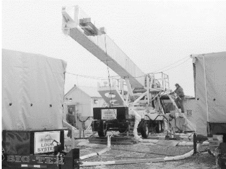
Figure 3. The Light Duty Utility Arm deployed various end effectors into tank WM-188 at the INEEL tank farm to take interior video and collect waste samples.
