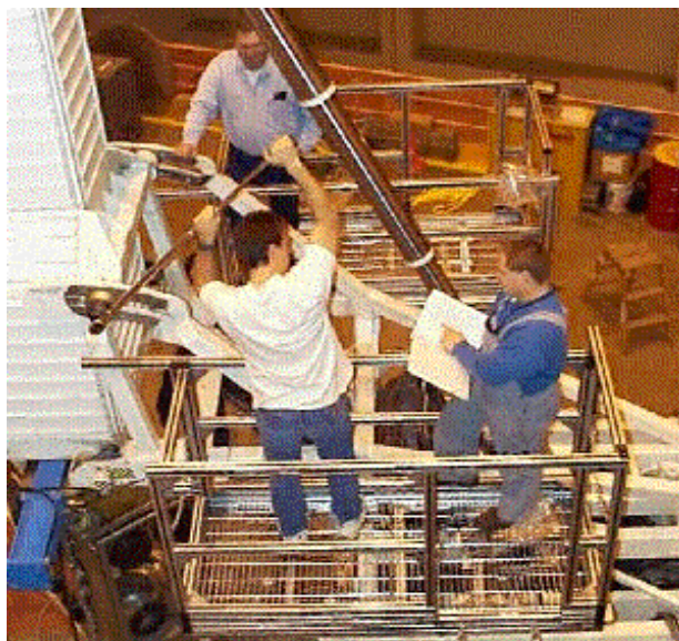
Figure 2. System operators trained using the LDUA in a cold-test facility prior to deploying it into underground storage tank
