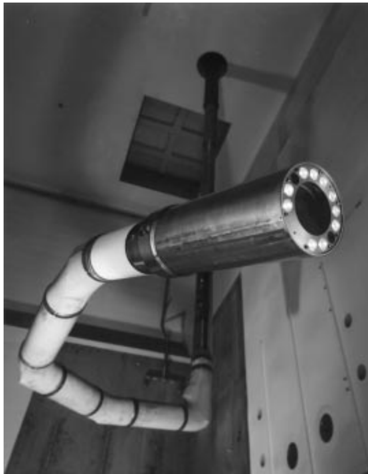
Figure 1. The Stereo Viewing System end effector uses video cameras that enable close up inspection of tank structures.
