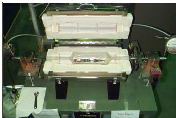
Figure 1. Bench-scale rotary calciner with quartz reactor.
