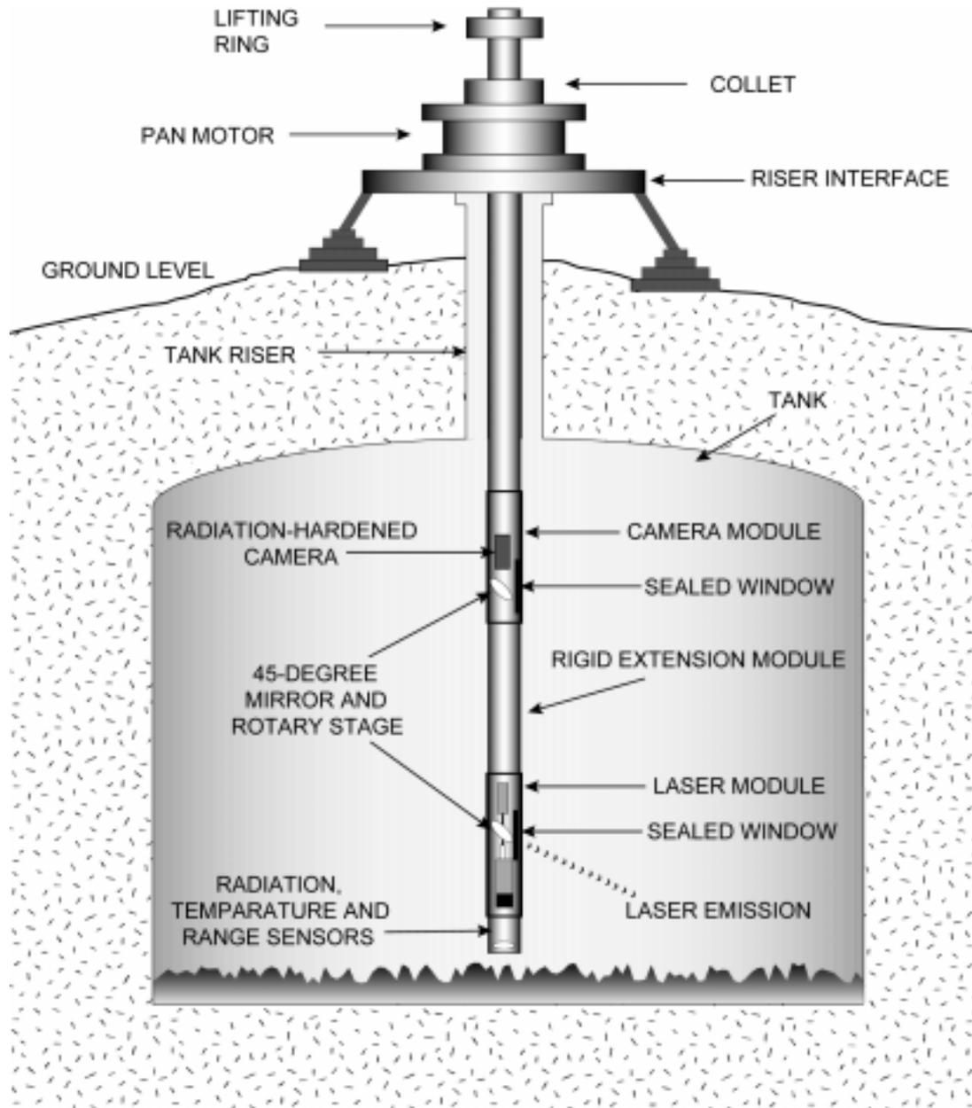
Figure B1. Configuration of the Topographical Mapping System as deployed in an underground storage tank (not to scale).
