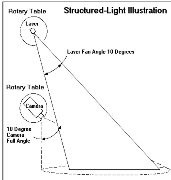
Figure 2. Structured light for range measurement.
