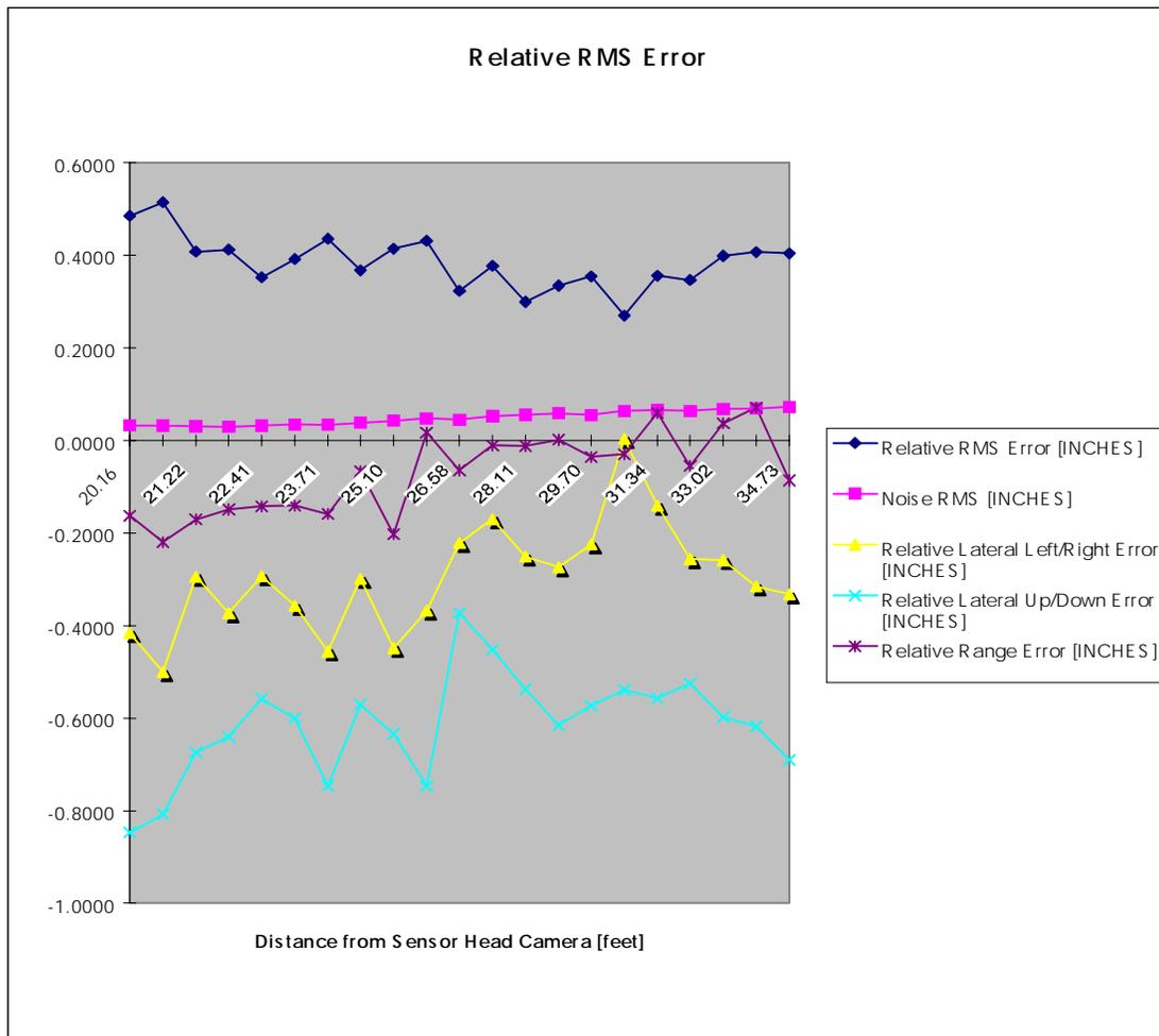
**Figure 3. Relative accuracy of the Topographical Mapping System.**
