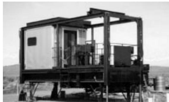
**Figure 1. Truck-mounted Vadose Zone Characterization System.**
