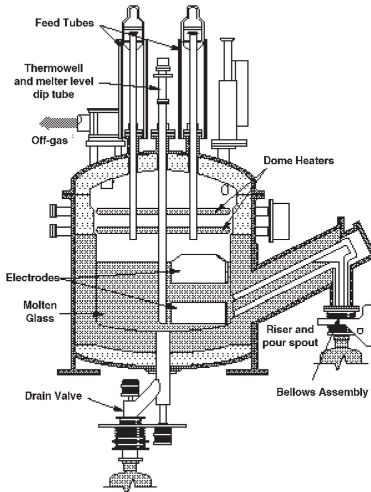
Figure 2. Joule-heated melter.
