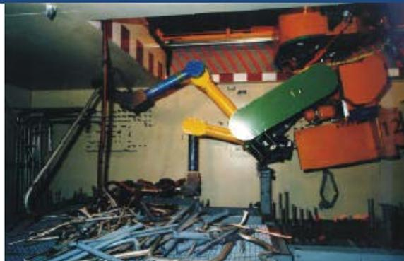
Horizontal remote crawler/digger tool; Vertical remote dismantling equipment
