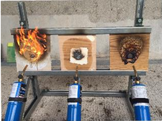
Fire resistant qualities of intumescent coatings (middle) compared to existing industry fixatives (left and right)
