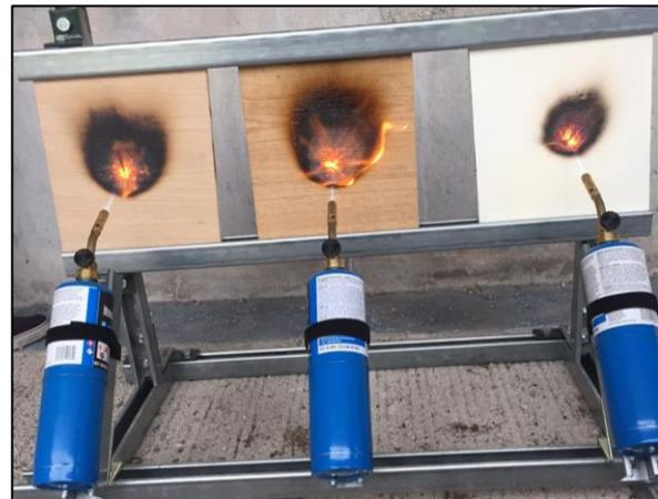
**At the 2-minute mark: wood only (left) and wood with a leading industry fixative (middle) began to show significant degradation and burn through when exposed to a direct flame. The wood with leading industry fixative layered with an intumescent coating (right) began to develop a thickening char from the expanding intumescent coating.**
